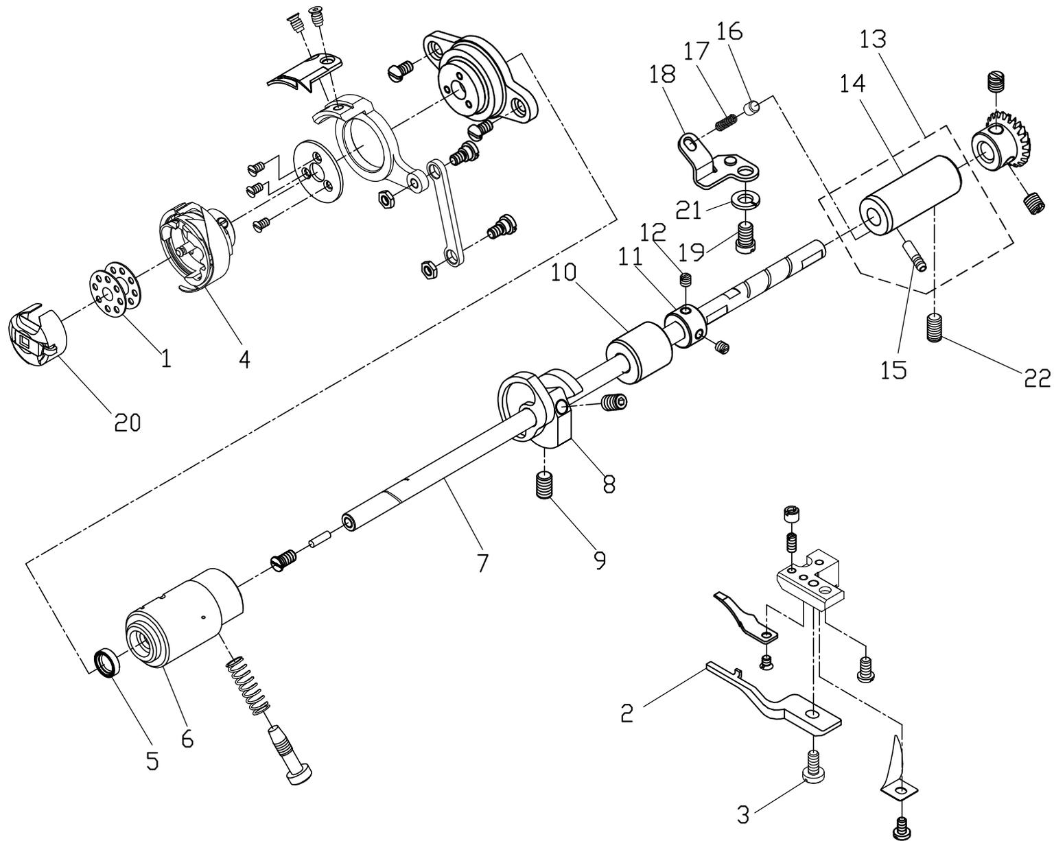
G. CS-5150-BT 下軸關係 LOWER SHAFT MECHANISM COMPONENTS
