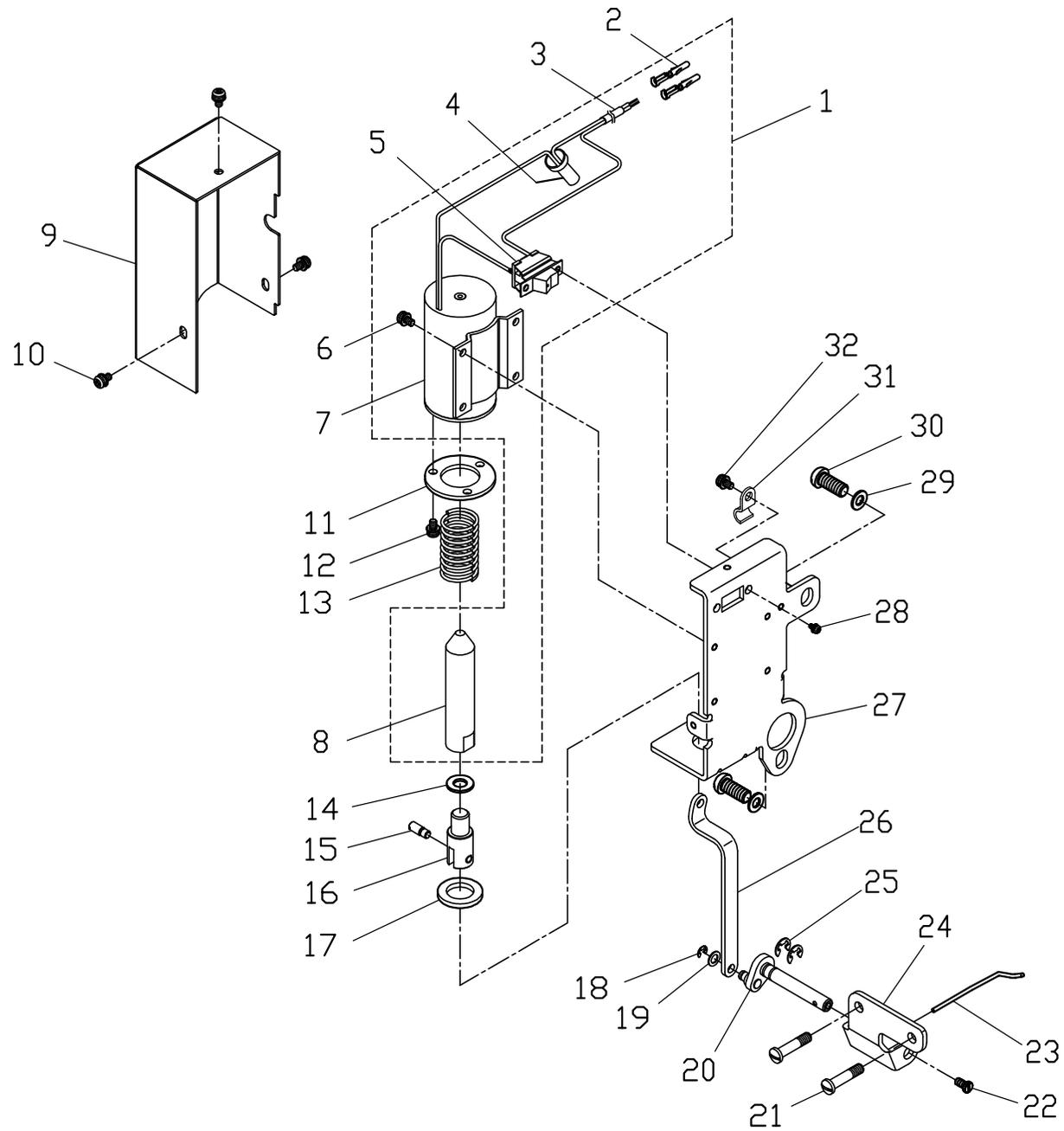
K. CS-5150-BT 撥線桿關係 WIPER MECHANISM COMPONENTS
