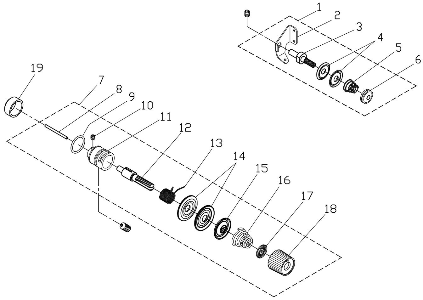
I. CS-5150-BT 縫線壓力調節關係 UPPER THREAD TENSION REGULATOR MECHANISM COMPONENTS
