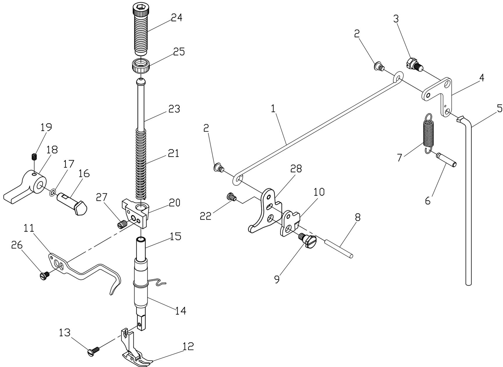
D. CS-5150-BT 押脚・脚弓関係 PRESSURE BAR & KNEE LIFTER COMPONENTS
