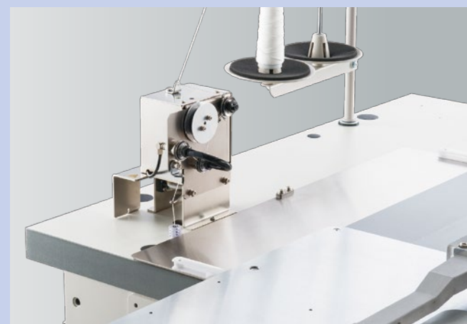
Constant-quantity bobbin thread feeding mechanism
