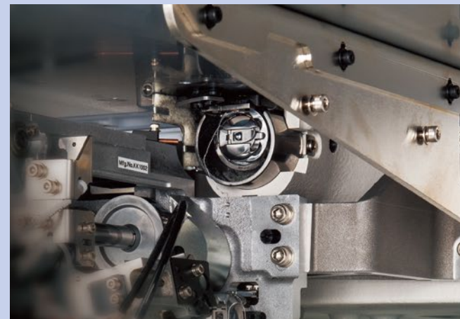
Automatic bobbin-thread winding and feeding unit
