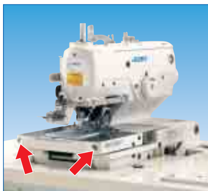
Material opening amount adjusting screw MEB-3200SS
